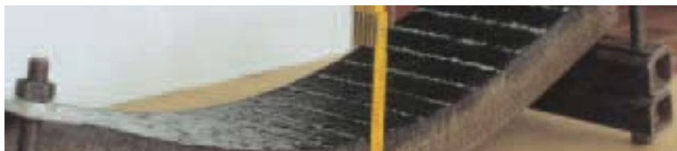
A laboratory test showing DAC flexing up to 50mm without showing signs of cracking and still retaining its impermeability
